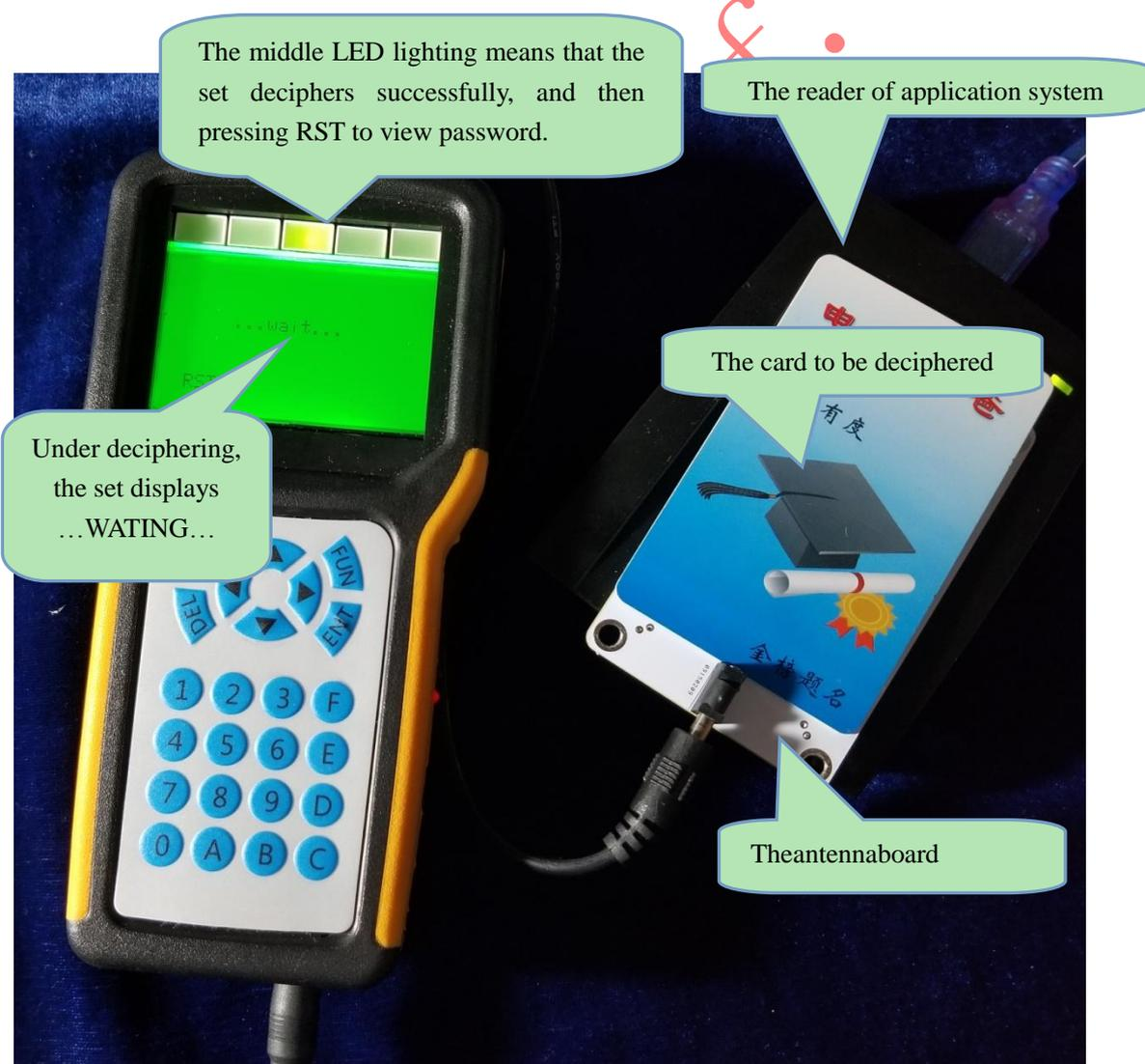
Fig2.4.5 The connection of deciphering password
