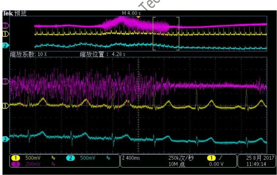
Where: wave 1 is V5 lead of ECG, wave 2 is V2 lead of ECG, wave 3 is bicipital muscle of arm, A and B and C channels.
